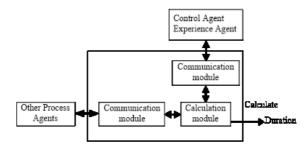
Fig. 8. the internal structure of the Process Agent and its communication relationship
